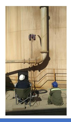
Technology in place - NDT Crawlers for thickness testing
